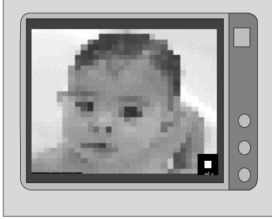
Figure 3-15. Flat panel display with a rectangular psf .
